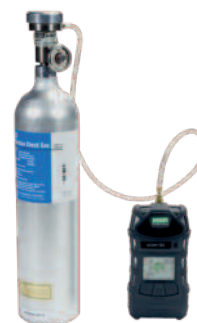
Manual Testing with Test Gas
