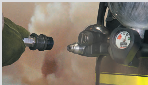
MSA's Quick-Fill® System allows workers to extend SCBA air supply by replenishing via a hose from a secondary air source, such as a cascade cylinder bank.
