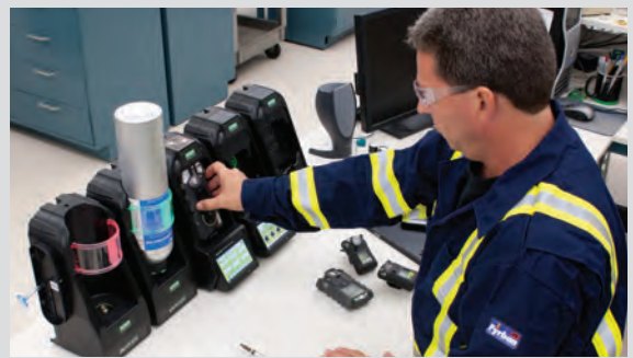
MSA's GALAXY® GX2 Automated Test System offers ease of use, reduced cost of ownership and proactive safety management. Integrated system provides simple and intelligent testing and calibration of MSA ALTAIR® product family.
