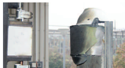
GS-ET-29 class 2-7 kA certification passed. Head and face combination protects the wearer.
