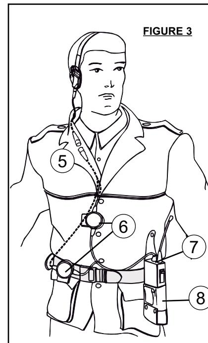
Connect the connection plug (7) to the transceiver (8) (set switched off).
