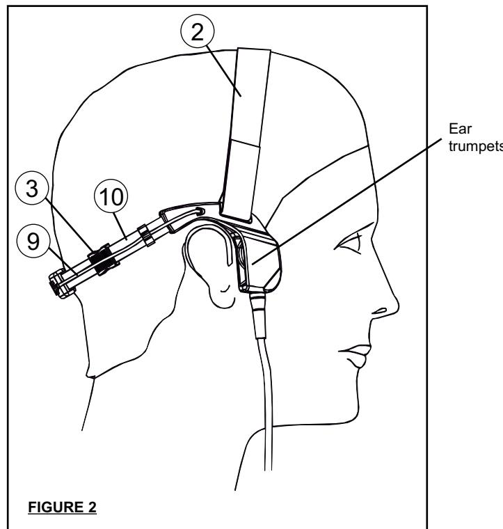
Place the equipment on the head as shown in figure 2. The harness (10) is in contact with the nape of the neck and the strap (2) goes over the top of the head. Adjust the size of the harness (2 telescopic half-harnesses) with the two buttons (3) so that the two ear trumpets lie flat on the side of the head.
