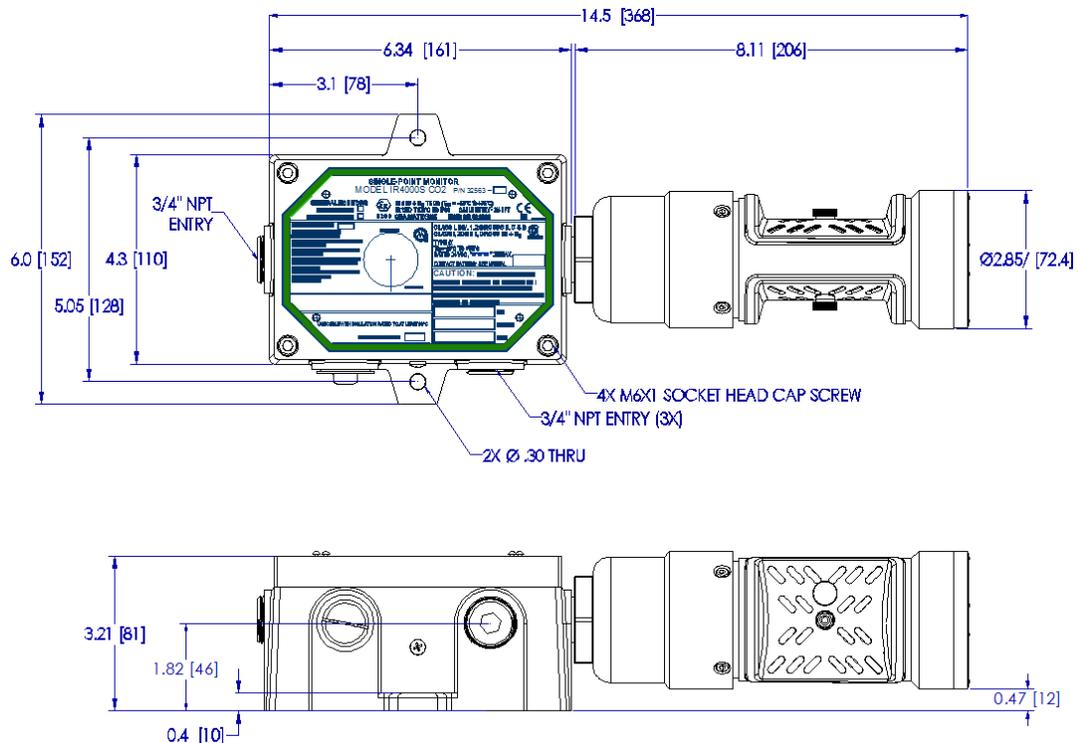
Figure 5. IR700 Mounting Dimensions
