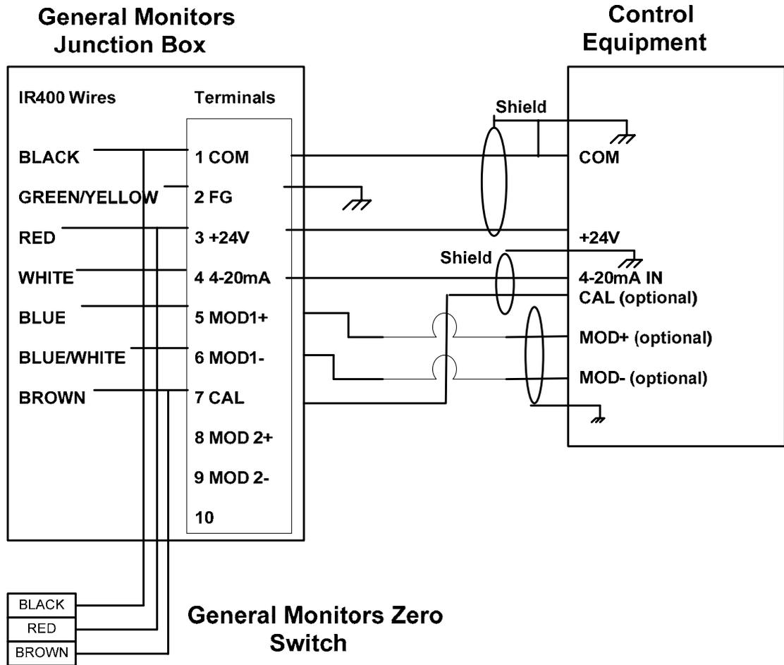
Figure 7: Wiring Diagram from IR700 to Control Equipment
