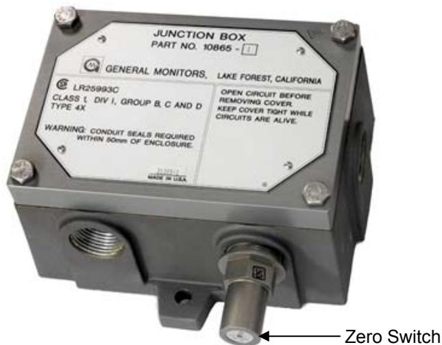
**Zero the Unit.** To insure a true zero and maintain IR700 accuracy, the IR700 must be purged with nitrogen for a sufficient time to remove all naturally occurring carbon dioxide. Apply the General Monitors magnet that was included with the unit to the Zero Switch / LED for approximately three seconds. The LED in the switch will light to show proper placement.
