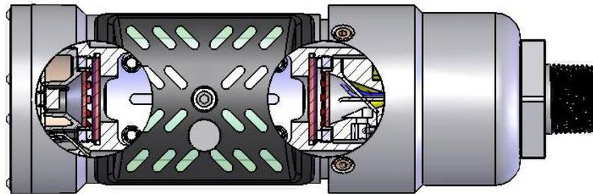
Figure 9. IR700 optical window locations
