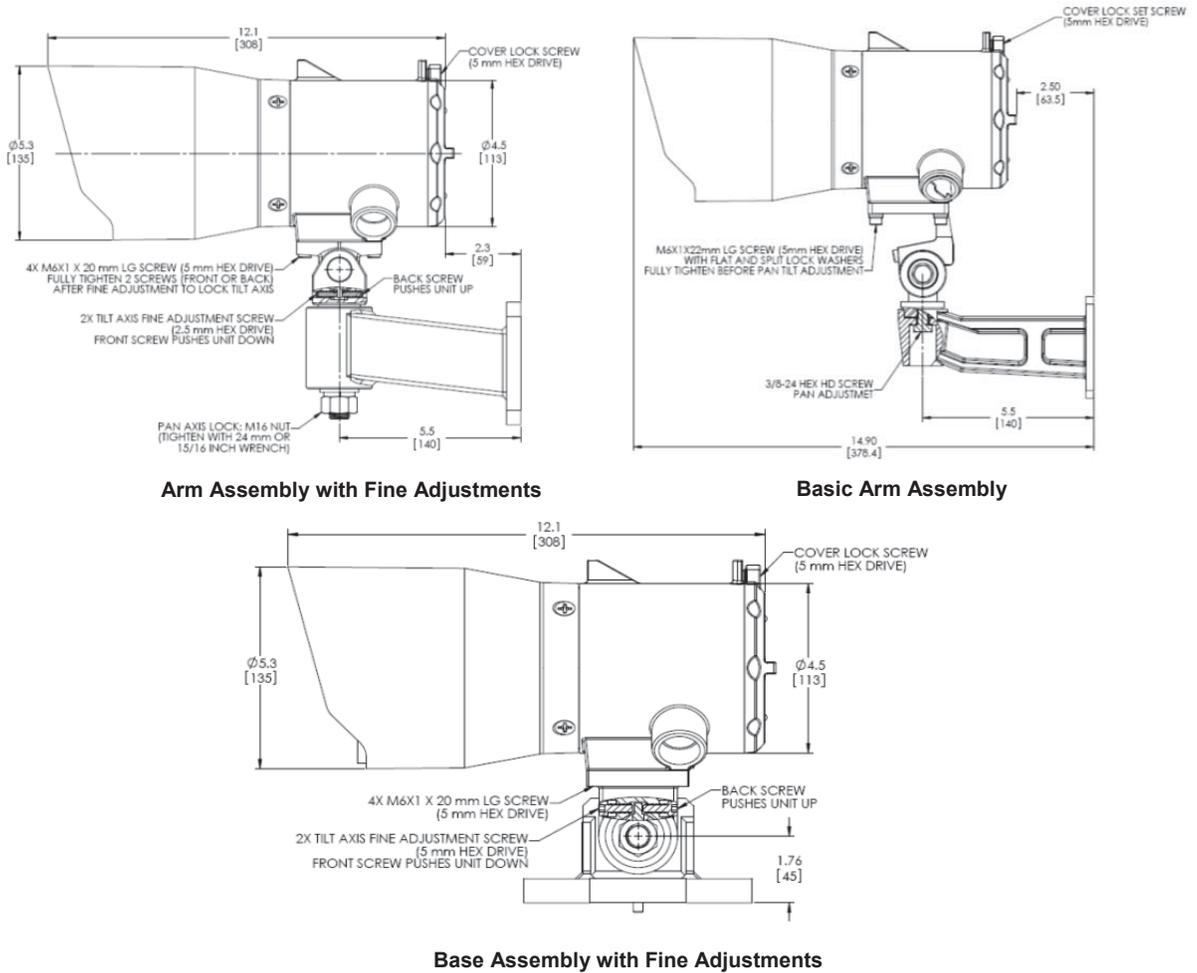
**Fig. 4 Outline and Dimensional Drawing with Mounting Options**
