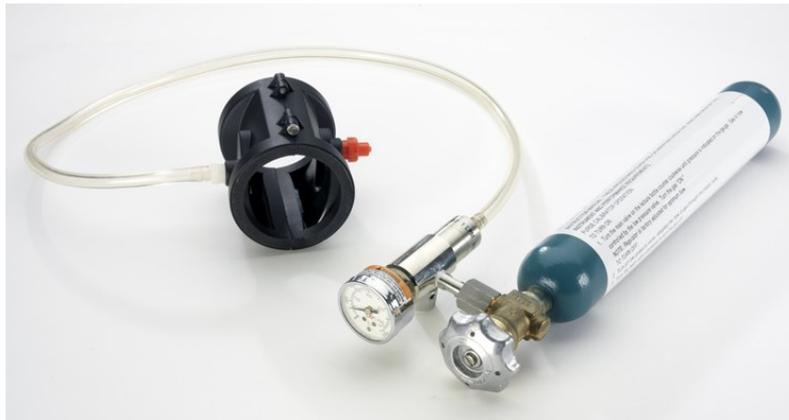
The portable purge calibrator is a compact, accurate and safe system containing a non-explosive gas concentration. The lecture bottle is filled with a standard 50% LEL mixture of gas/air. Using a known gas/air mixture reduces the likelihood of error in field calibration.
