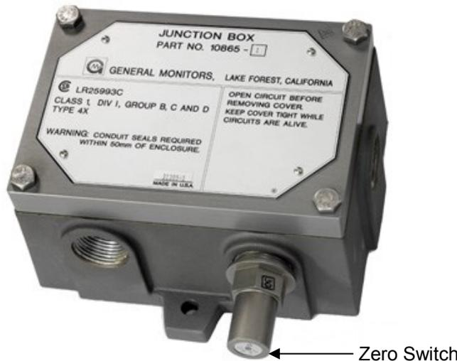
**Zero the Unit.** Apply the General Monitors magnet that was included with the unit to the Zero Switch / LED for approximately three seconds. The LED in the switch will light to show proper placement.
