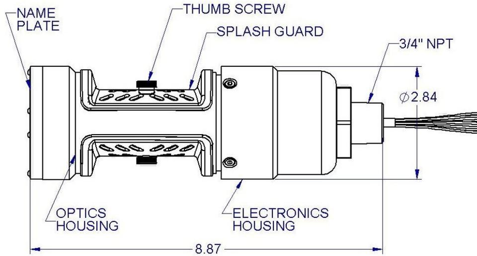
**Figure 9: Outline and Dimensional Drawing, IR400, Inch Measurements**
