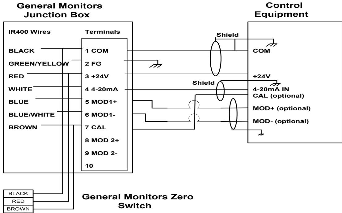
Figure 6: Wiring Diagram from IR400 to Control Equipment
