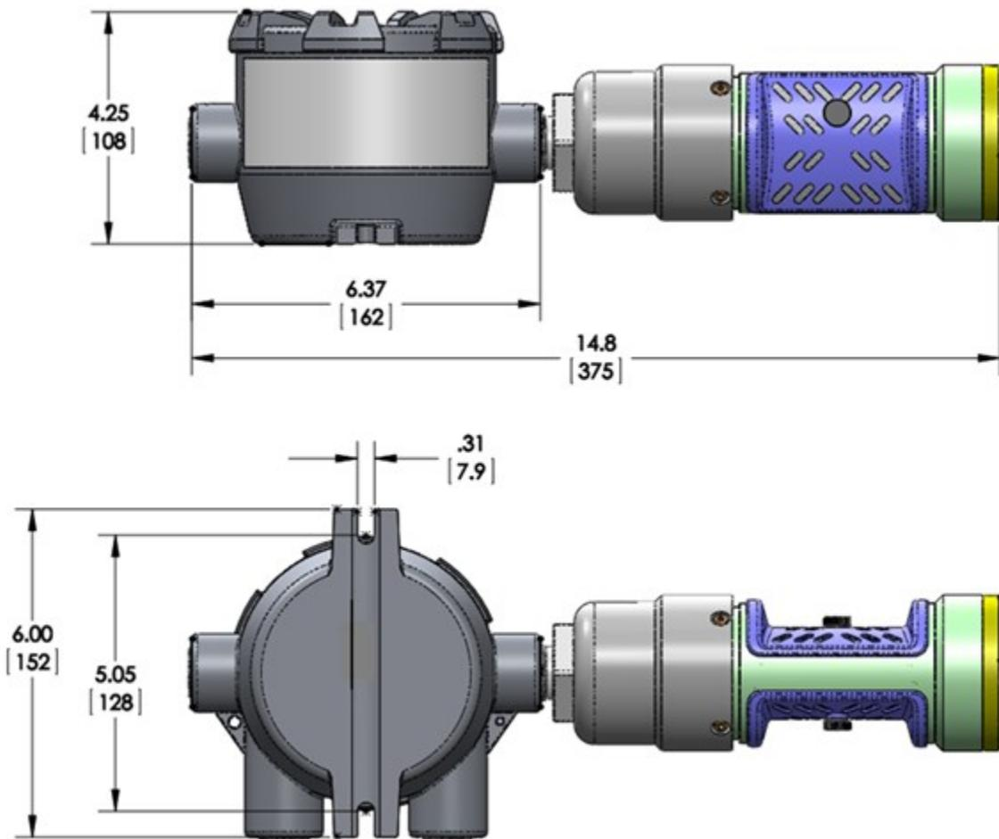
**Figure 5: Dimensions for IR400 mounted with S5000 Gas Monitor**
