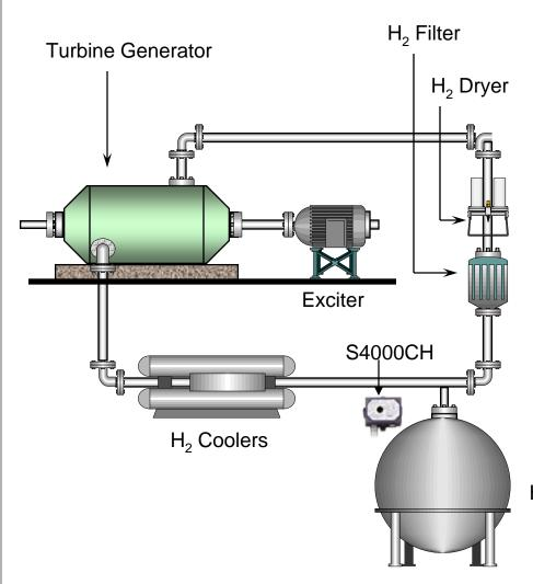
Because of its ideal cooling properties, hydrogen is used in power plant generators.
