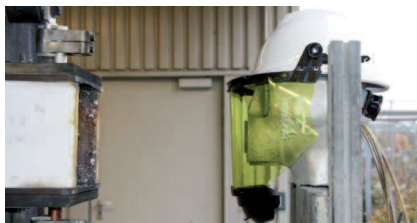
MSA vlamboogset vóór "boog-in-box-beproeving" 7 kA
