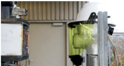
MSA arc flash set before "arc-in-the-box testing" 7 kA
