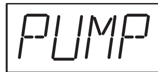
PUMP – Pump Failure
