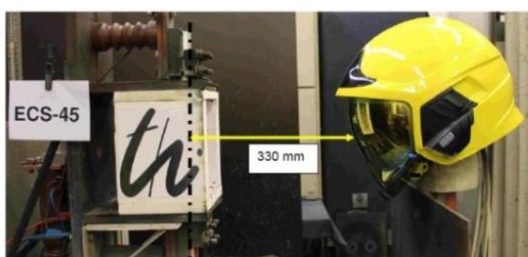
Figure 2. Test set-up with helmet visor combination
