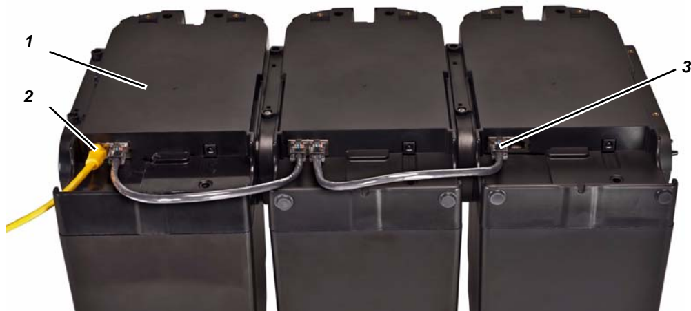
Fig. 11 Test Stand Ethernet connections
