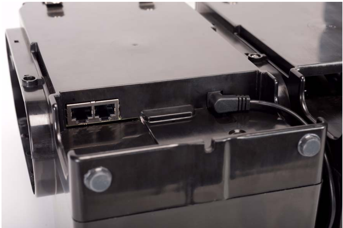
Fig. 6 Test Stand Ethernet jacks
