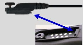
**Step 4.** Insert the USB end of the cable in the computer that is running RPM2.
