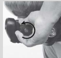
**Step 4.** Begin breathing (with the regulator attached) and the radio and SCBA will connect automatically (approx. 20 seconds).
