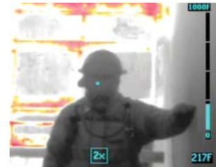
Same picture with 2X Digital Zoom activated showing Low-Sense imagery on the display of an E5200HD 2 TIC
