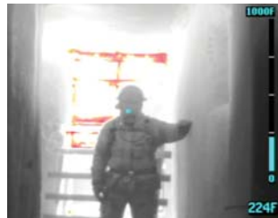
Low Sense imagery on the display of an E5200HD 2 TIC
