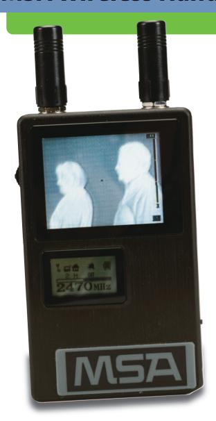
MSA's compact Wireless Handheld Video Receiver is a frequency-scanning analog receiver well suited for law enforcement, security, and surveillance use. It will pick up images from any video transmission source in the scanning frequency range, including MSA's ThermalTrac™TIC when the TIC is equipped with the video transmitter described on the reverse of this page.
