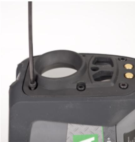
*Figure 19 Germanium lens retainer, screws to be removed*
