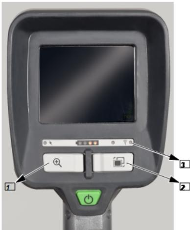
Figure 9 Additional buttons EVOLUTION 6000+ TIC and 6000 X TIC
