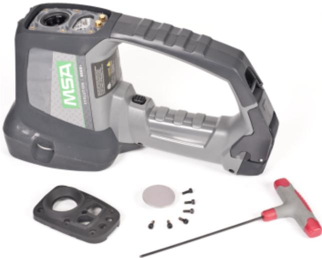
*Figure 18 Germanium lens retainer, parts and tools*
