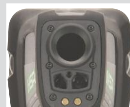
Field-replaceable germanium lens
