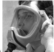
and repeat steps 1 and 2. If you cannot maintain a seal by adjusting the headstraps, check the facepiece for leaks. Locate the problem and correct it before using the respirator.
