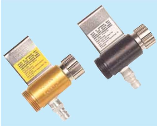
High-pressure control valve is designed to deliver the required air flow to the facepiece at an inlet pressure range of 35-40 psig for hose lengths of 8 to 300 feet. Low-pressure control valve is designed to deliver the required air flow to the facepiece at an inlet pressure range of 10-15 psig for hose lengths of 8 to 50 feet. The valve includes an integral belt clip and male and female quick-disconnect assemblies. (See back page for parts information chart).
