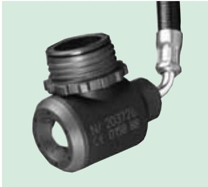
The LA 88-N is a normal pressure lung governed demand valve in a specially small and lightweight design. A servo-control controls the air flow. The pivotable medium pressure line adjusts very well to head movements, so that the user is not encumbered. The connection to the mask is a handwheel with thread according to EN 148-1 [standard thread].
