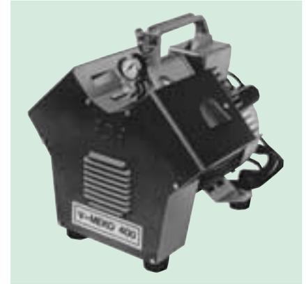
The Diaphragm Compressor V-Meko 400 is a small, portable compressor with an intake performance of 360 l/min and a medium pressure of approx. 5 bar. The compressor supplies oil-free air, eliminating the need for additional filters.
