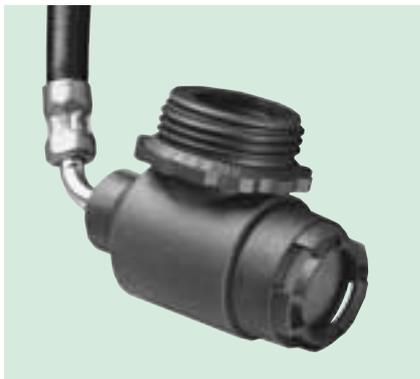
The LA 88-AE is a small, light-weight positive pressure lung governed demand valve, which automatically switches to positive pressure with the initial breath. By pushing the large, red button on the side, it can be switched again to normal pressure to avoid loss of air when removing the apparatus. The pivotable medium pressure line adjusts very well to head movements, so that the user is not encumbered. The connection to the mask is a handwheel with thread according to EN 148-3 [M 45 x 3].
