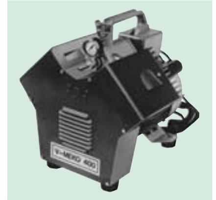
The Diaphragm Compressor V-Meko 400 is a small, portable compressor with an intake performance of 360 l/min and a medium pressure of approx. 5 bar. The compressor supplies oil-free air, eliminating the need for additional filters.
