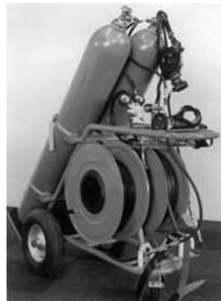
The **Air Cart 2 x 50 l** is especially designed for long-duration work. It is equipped with a pressure reducer with high and medium pressure gauges, safety valve, warning signal, medium pressure coupling and a Y-piece.
