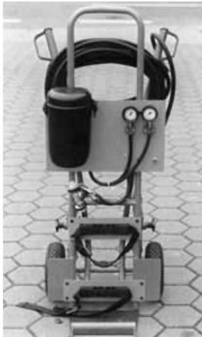
The **Air Cart 2 x 6 l** is a breathable air supply system which is not restricted to a specific location. It is designed for two 6 l/300 bar, resp. 6.8 l/300 bar compressed air cylinders.
