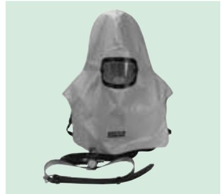
The Sandblast Cap Light consists of a silicone full face mask with large lens, a replaceable plastic cover lens and a sieve lens as protection against rebounding grit. The full face mask is firmly connected with the protective hood which covers the shoulders and chest area. Air is supplied to the mask from a pressure control with pressure gauge which is fixed to the waist belt. The silicone mask is comfortable to wear also for longer durations.
