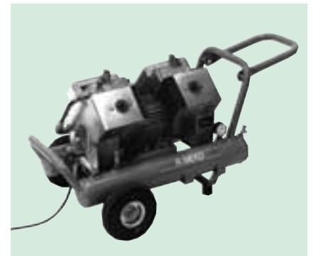
The Diaphragm Compressor R-Meko 720 has a 400 V motor and an intake performance of 720 l/min. The compressor is fixed onto a solid frame with wheels so that it is not restricted to a specific location.
