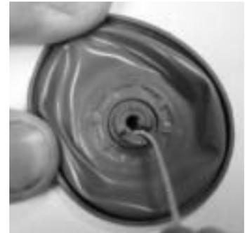
2. If the cuts are not completely through the center of the diaphragm nipple, do not use the diaphragm. MSA will replace diaphragms that do not have three distinct slits in the diaphragm nipple.
