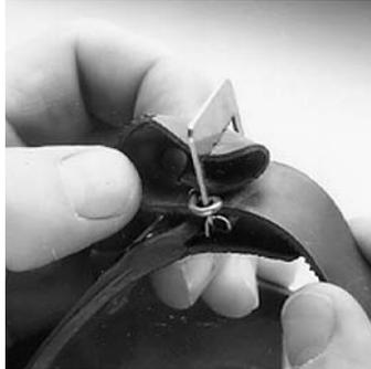
2. To install a new rubber headstrap, lay the new headstrap flat. The MSA logo should be right-side up. The strap is labeled. Pick the headstrap up by the strap labeled "FRONT."
