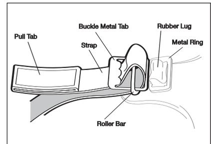
**Note:** It is important to have the folded side of the elastic strap face up, so the strap will lay flush against the head when it is pulled tight.
