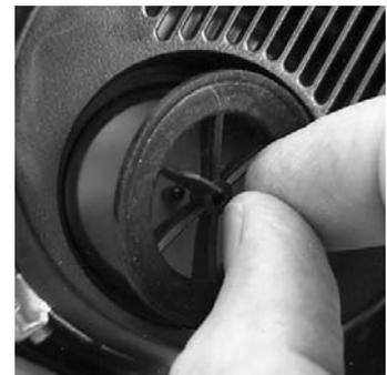
4. Remove the valve disc from the coupling nut housing. If you cannot grasp the disc with your fingers, use a blunt object, such as a ballpoint pen to lift one edge, then remove the disc. Be careful not to tear the soft disc.
