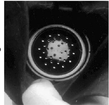
Be sure that the crimped side of the speaking diaphragm is facing up (away from the gasket or o-ring).
