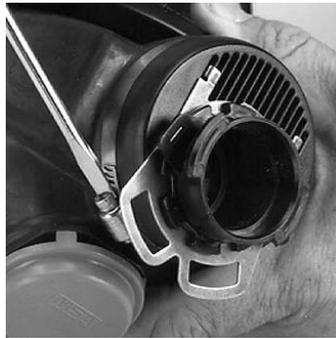
e. Tighten the band clamp until the inlet is secured. Be sure that the band clamp will not pull the facepiece rubber away from the assembly. Do not over-tighten. If the facepiece rubber "bulges" out through the slots in the clamp, the clamp is too tight and must be loosened and re-tightened.
