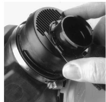
c. Be sure that the assembly is pressed into the facepiece completely.
