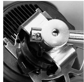
2. Lift the neckstrap retaining ring off the housing. Note how the "fingers" line up in the housing.
