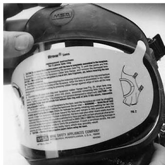
Then insert the lens into the groove. Work the facepiece flange around the lens to seat the lens fully in the groove.
