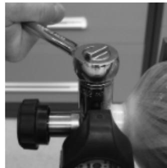
2. Discard the safety nut, gasket, and pressure disc.
