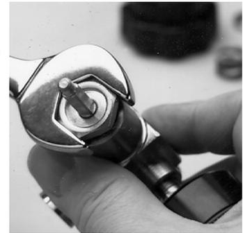
4. Pull the packing gasket out of the valve body.
