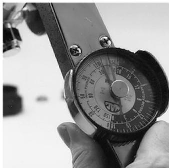
6. Place the handwheel on the stem and check the valve for proper motion. The handwheel should move freely. Now turn the handwheel clockwise to close the valve. Once closed remove the handwheel and tighten the packing gland to 85 - 110 in-lbs. Once completed place the handwheel back onto the stem and open the valve fully.
