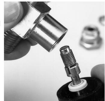
**Note:** If the insert shows signs of wear or damage it must be replaced.
