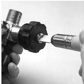
2. Also remove the spring and lift the handwheel off the valve stem.
