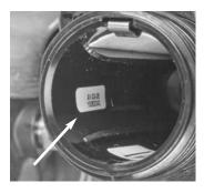
On the FireHawk M7 Power Module, the label can be found inside the battery tube by removing the battery cap.
