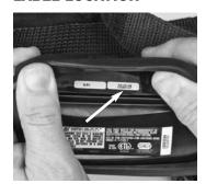
On the FireHawk M7 Control Module, the label can be seen by pulling back the rubber boot on the side opposite of the yellow reset button.
