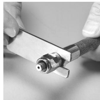
3. The hose must be replaced by an MSA Certified Air Mask Technician with a new Hose Assembly P/N10004650.
