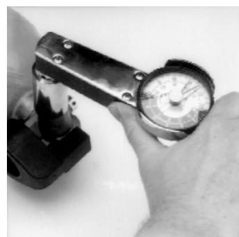
5. Turn the valve stem counter-clockwise until the stem stops. Be sure the gland does not turn.
