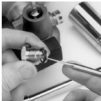
**Note:** The O-ring removal tool can be used to remove O-ring from the packing gland.
