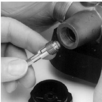
**Note:** If the insert is white or shows signs of wear or damage it must be replaced.
