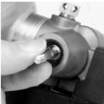
4. Replace the handwheel on the valve stem. Turn the stem until the slot drops onto the insert. Turn the handwheel counter-clockwise until the insert can be removed.
