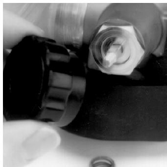
2. Place a 7/8" socket (deep-well) on the packing gland flats. Unscrew the packing gland from the valve body. Pull the stem out of packing gland. Remove the O-ring and valve stem washer from the packing gland.
