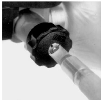
11. Open and close the valve completely several times to seat the stem, insert, and the valve stem gasket.
