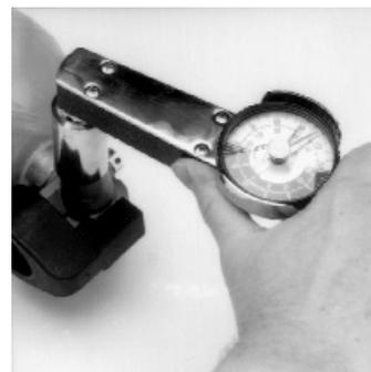
7. The valve stem square must fit into the square hole in the handwheel. Place the handwheel on the stem and check the valve for proper motion. The handwheel should move freely.
