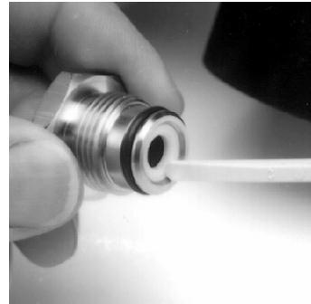
3. Place a new washer into the packing gland. Press the washer down to its seat.
