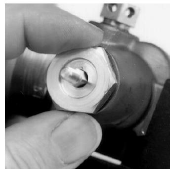
4. Insert the stem into the valve body. Turn the stem until the slot drops onto the insert. Thread the packing gland into the cylinder valve until it is finger tight.
