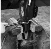
2. Slide a wrench over the iam nut and loosen by turning the wrench counter-clockwise.
