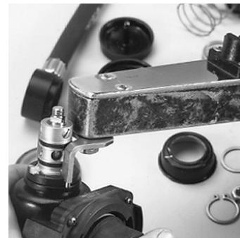
6. **Place two drops of urethane adhesive (P/N 603571)** on the exposed threads of the valve core. Do not permit thread sealant to contact the regulator housing.
