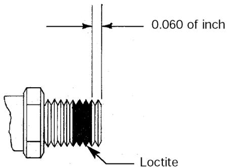
3. Thread ICM unit in to Quick Fill Block until it stops. The Quick-Fill Block must be oriented with the coupling as shown in the figure below. To obtain this alignment. Unthread ICM unit not more than one full turn. Hold the ICM unit to prevent turning. Tighten the new jam nut against the Quick Fill Adapter Block and torque to 200 - 225in.lbs with a thin crowsfoot wrench.
