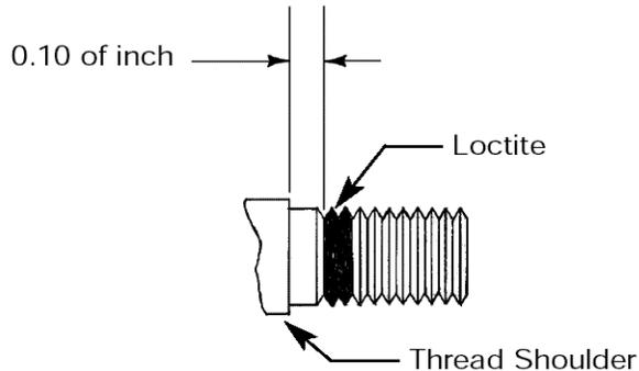
2. Thread the NEW jam nut (P/N 10003606 Dull Surface Finish) against the thread shoulder of the ICM unit. Apply Loctite 271 to three threads approximately one-sixteenth (0.060) of an inch from the end of the ICM unit.
