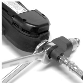
3. Unthread ICM unit from Quick Fill Adapter Block.
