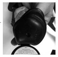
3. Carefully remove black gauge plug using Plug Disassembling Tool (P/N 10146831).
