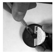
4. Wipe the recessed sur face with a clean, dry cloth to remove any debris.
