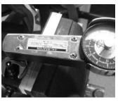
NOTE: The crowsfoot must be perpendicular to torque wrench.
