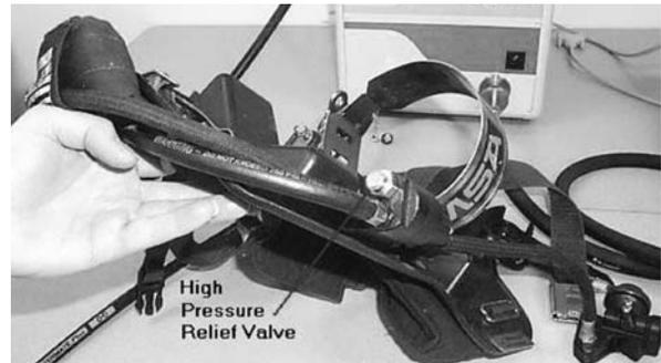
Locate and remove the first stage regulator safety relief valve.
