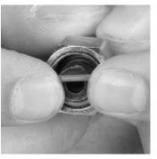
c. Use the o-ring removal tool to slide the o-ring into the groove.
