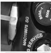
(1) Apply leak test solution to the union between the cylinder valve fitting and the valve body.
