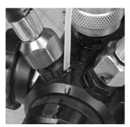
(1) Apply leak test solution to the union between the hose adapters and the valve body.
