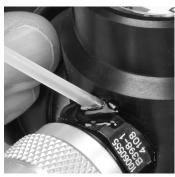
(2) Apply leak test solution to the union between the fill port and the valve body.
