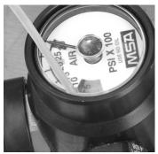
(1) Apply leak test solution to the union between gauge bezel and the valve housing.
