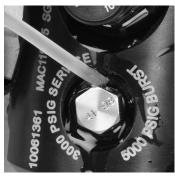
(2) Apply leak test solution to the union between the plug and the valve body.
