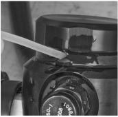
(1) Apply leak test solution to the union between the regulator cap, seal ring and valve body.
