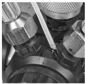
(2) Apply leak test solution to the hose connections.
