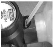
(2) Apply leak test solution to the union between the cylinder adapter and valve body.
