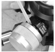
(1) Apply leak test solution to the union between the fill port cap and the fill port.
