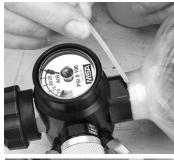
(1) Apply leak test solution to the cylinder neck.
