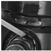
(1) Apply leak test solution to the union between the relief valve and the valve body.
