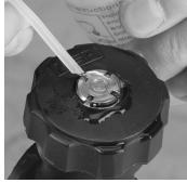
(2) Apply leak test solution to the locknut.
