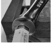
(3) Use the 5/8" wrench to disconnect the check valve from the quick connect.
