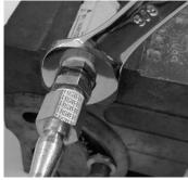
(3) Use the 5/8" wrench to disconnect the check valve from the filter.
