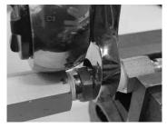
(4) Use the 5/8" crowfoot and foot-pound torque wrench to tighten the check valve onto the quick connect to  $10 \pm 2$  ft-lbs.
