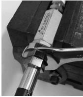
(3) Use the 11/16" wrench to disconnect the hose from the filter.
