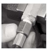
5. Use an 11/16" crowfoot and foot-pound torque wrench to tighten to no more than 25 ft lbs.
