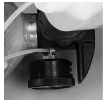
3. If bubbles appear, replace the pressure gauge and test again. (See **AirHawk II Cylinder and Valve Maintenance and Repair** for instructions.)
