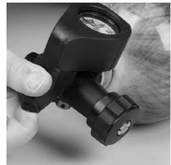
2. Apply leak test solution to the pressure gauge stem, cover, and bezel.
