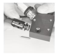
4. Use the **o-ring removal tool** to remove the oring.
