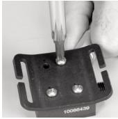
Installing the Screen and Screen Retainer Screen 10048620
