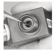
2. Turn the Work-Line assembly over and allow the screen to fall out.
