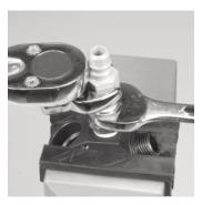
**NOTE:** For plug, P/N 55716, use an inch-pound torque wrench and 5/8" crowsfoot or socket to tighten the plug to 96-112in.lbs. This applies to Work-Line Assembly P/N 10086442.
