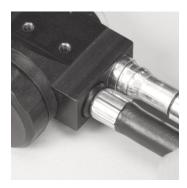
Reinstall the PR14 First Stage Regulator. (See AirHawk II PR14 First Stage Regulator Maintenance and Repair, P/N 10104220 for instructions)
