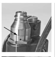
...or at the joint where the coupling attaches to the air mask, remove the air mask from service until a replacement coupling is installed.
