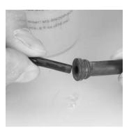
2. Lubricate the barb with Snoop (P/N 600920) and push the drinking tube onto the drinking tube connector ½".
