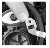
3. Pull the lens out of the groove.
