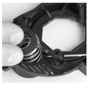
b. Lift the pneumatic retainer out of the component housing cover.
