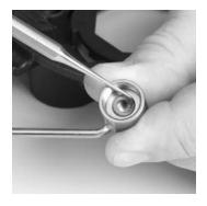
e. Install the pneumatic nut. Use the inch pound torque wrench, ¼" socket, and Pneumatic Nut Special Tool (P/N 10086032) and tighten to 8 in lbs.
