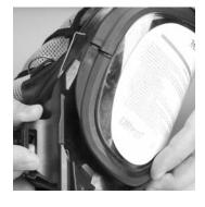
3. Align the screw hole in the lower metal tab with component housing screw hole.
