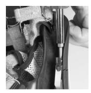
Remove the component housing cover. (See Removing the Component Housing Cover for instructions.)
