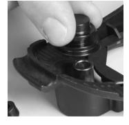
f. Use the o-ring removal tool to remove the o-ring.
