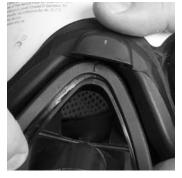
3. Align the component housing ring center mark with the facepiece centerline. Lubricate with Snoop (P/N 600920) as needed.
