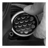
2. Install the retaining ring (P/N 804808) and firmly hand tighten.
