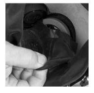
Unscrew and remove the speaking diaphragm retaining ring.
