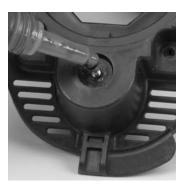
b. Use the inch pound torque wrench and 5/16" socket to tighten the nut to 6 in lbs.
