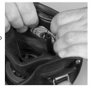
b. Stretch the nose cup over the retaining ring.
