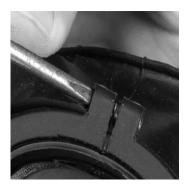
a. Make sure the facepiece rubber does not extrude between the component housing ring ends.
