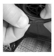
4. Start at the narrow end and work the housing ring onto the facepiece. a. Work down both sides until the ring completely captures the facepiece rubber. Lubricate with Snoop (P/N 600920) as needed.
