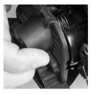
**Note:** Be careful not to lose or damage the exhalation valve spring.
