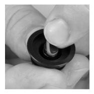
2. Assemble the exhalation spring onto the piston.
