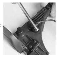
Use a Phillips screwdriver to tighten the component housing ring screw.
