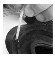
7. Lubricate the lens ring with Snoop (P/N 600920).
