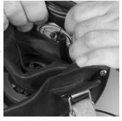
c. Stretch the nose cup over the retaining ring.
