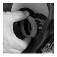
8. Remove the ClearCommand microphone.
