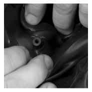
b. Stretch the nose cup over the exhalation valve flange.
