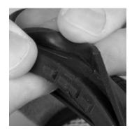
Lubricate the groove with Snoop (P/N 600920) or properly mixed Confidence Plus cleaner sanitizer solution.
