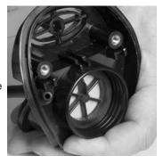
Pull drinking tube connector out of internal drinking tube.
