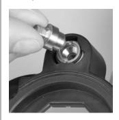
d. Remove the pneumatic tube.
