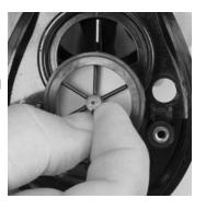
**Note:** Ensure that the groove captures the component housing rim. Flex the gasket spider as needed to fully capture the rim. When installed correctly, the gasket lays flat and all of the spokes are straight.
