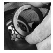
3. Carefully remove the speaking diaphragm.
