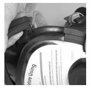
a. Make sure that tab is under the lower lens ring.
