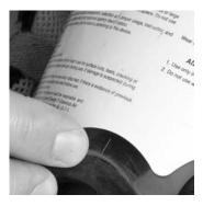
Moisten the mating surfaces of the facepiece and lens ring with Snoop (P/N 600920).
