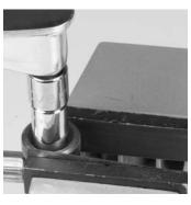
d. Screw the bypass assembly into the valve assembly.
