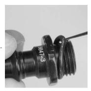
**NOTE:** Be careful not to scratch the o-ring groove. Discard the o-ring.
