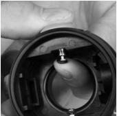
**NOTE:** Install the thicker o-ring (P/N 10037951) inside the housing.
