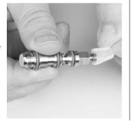
e. Spread a thin layer of Christo-Lube to the end of the bypass threads that go into the housing.
