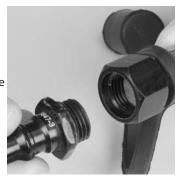
Use a 3/4" wrench to hold the hose union and a 3/4" crowfoot and inch pound torque wrench to tighten the nipple to 75 ± 5 in lbs.
