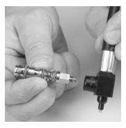
NOTE: To prevent damage to the o-ring, use extra caution when installing the bypass assembly. Check for evidence of o-ring damage before proceeding. O-ring damage may be visible through u-clip openings. Replace damaged o-rings.
