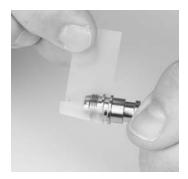
c. Slide the silicone o-ring over the protective paper or tape.
