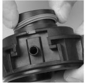
NOTE: An unseated seal ring can cause an air leak.
