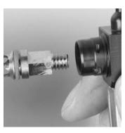
7. Turn the bypass manifold upside down and allow the bypass stem to fall out.
