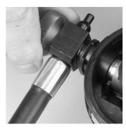
4. Secure the bypass knob in a vise.
