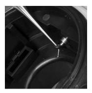
b. Pull firmly on the buttons to remove them. Be careful not to lose the springs.
