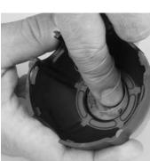
1. Install the spring into the cover. Ensure that the last coil is captured by the regulator cover tabs.
