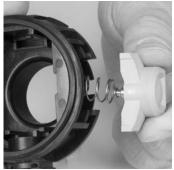
c. Remove the old orings. Be careful not to scratch the o-ring grooves. Discard the orings.
