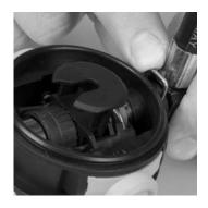
NOTE: Replace the Spring Cap (P/N 10047528) and Tetraplex CBRN Shield (P/N 10044026) per overhaul frequency. (See FireHawk® M7 Air Mask Maintenance and Repair, Introduction (P/N 10093079) for required overhaul frequency.)
