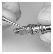
Removing the Bypass Screen
