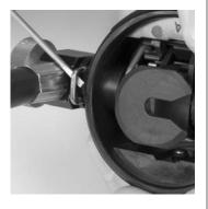
3. Unscrew the bypass assembly and pull the bypass assembly and housing from the valve housing.
