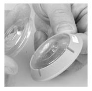
2. Roll the edge of the diaphragm off the lip of the regulator housing.
