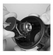
2. Push the valve into the regulator housing.
