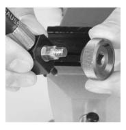
6. Gently pull the bypass assembly from the bypass housing.
