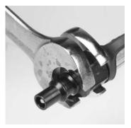
2. Use the o-ring removal tool to remove the oring.
