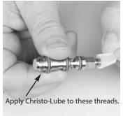
3. Carefully install the bypass assembly.
