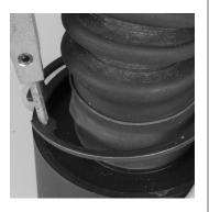
2. Pull the breathing tube from the breathing tube housing.
