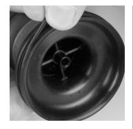
**Note:** Take care to securely grip the snap ring to avoid damage. Replace damaged or broken spring clips.
