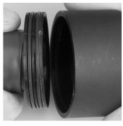
**Note:** Visually inspect to ensure o-rings are not cut or moved out of the grove. If o-rings are cut or moved out of groove, discard the o-rings and start again.
