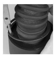
Carefully push the breathing tube into breathing tube housing.
