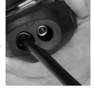
5. Stretch the new boot onto the Control Module housing.
