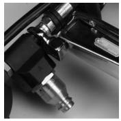
b. Turn the Jam Nut counterclockwise until it is butting against the connector.
