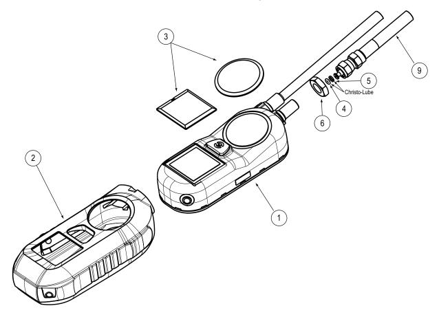
FireHawk M7 and FireHawk M7XT Control Module with Quick-Fill System
