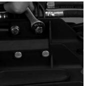
**Note:** Use extra care when disconnecting the power and data cable to avoid damage to the pins or socket.
