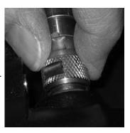
4. Use a torque wrench and **thin 9/16**" **crow foot** to tighten the connector to **10 in lbs.**
