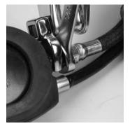
6. Use a **5/8" crow foot** to tighten the Jam Nut to **225 - 250 in lbs.**
