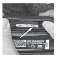
On the FireHawk M7 Power Module, the label can be found inside the battery tube by removing the battery cap.
