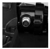
3. Hand tighten the connector until the o-ring is no longer visible.
