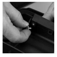
Use a slot head screwdriver to tighten the Friction Pad screws.
