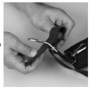
c. Pass the strap over the bar and back through the buckle.
