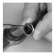
2. Pull the first stage intermediate pressure hose through the shoulder strap.
