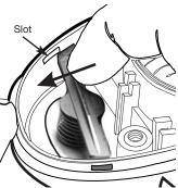
toward the bottom of the housing until the retainer snaps into slot.
