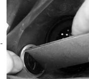
4. Unscrew and remove the retaining nut. Then, grasp the valve cover and gently pull the valve out from the underside of the facepiece.
