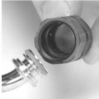
7. Remove the hose assembly O-ring. Be careful not to scratch the O-ring groove.
