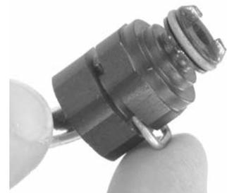
8. Slide the red bypass handwheel over the bypass body. The handwheel hex lines up with the handwheel.
