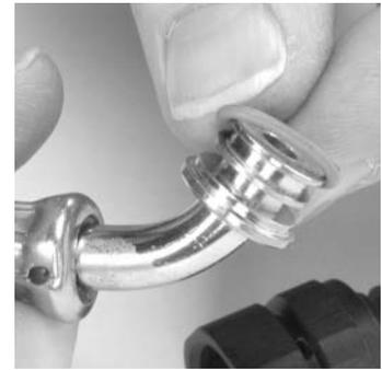
5. Apply a thin film of Christo-Lube lubricant (P/N 604070) into the second groove of the hose swivel.
