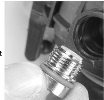
7. To remove the valve, turn the regulator housing upside down, or lift the valve out of the regulator housing.
