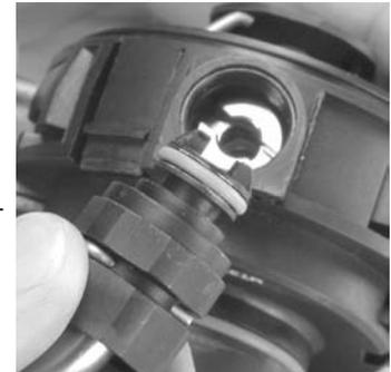
5. Turn the valve counter-clockwise to unthread the bypass insert from the valve.
