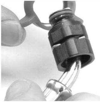
5. Using a screwdriver, remove the U clip from the bypass body.
