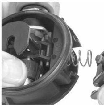
2. Pull on the buttons to remove them from the regulator housing. Be careful not to lose the spring.
