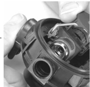
8. Replace all O-rings on the bypass insert and bypass body.
