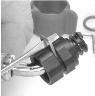
6. Remove the hose assembly by pulling the hose out of the bypass body.
