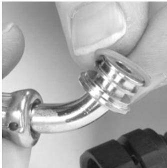
8. Inspect the second groove of the hose swivel. If dirty, all dirt and foreign matter must be removed before reassembling the bypass body.
