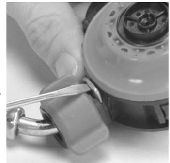
3. Remove the bypass and hose assembly from the regulator housing.
