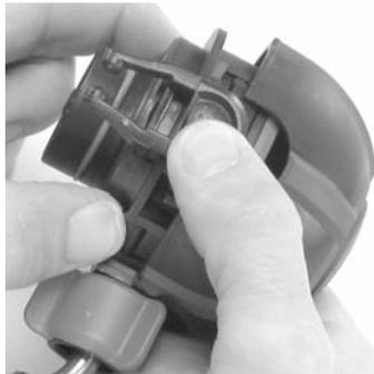
2. Pull firmly on the regulator cover to remove the cover, spring, and spring retainer from the regulator housing.
