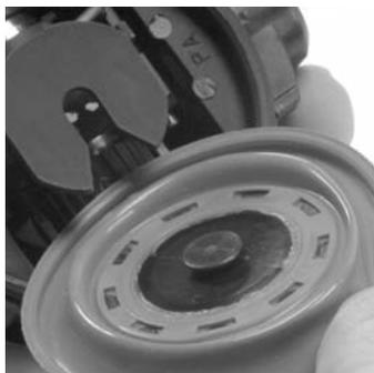
2. Roll the diaphragm edges over the regulator housing groove.
