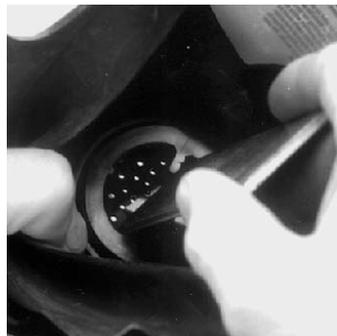
2. Turn the facepiece upside down and shake out the metal speaking diaphragm.
