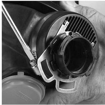
e. Tighten the band clamp until the housing is secured. Be sure that the band clamp will not pull the facepiece rubber away from the assembly. Do not over-tighten. If the facepiece rubber "bulges" out through the slots in the clamp, the clamp is too tight and must be loosened and re-tightened.
