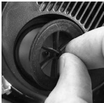
3. Lift the spider gasket out of the coupling nut housing by its tab.
