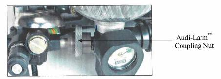
The design of the coupling nut joint allows the o-ring to compress before metal to metal contact prevents further tightening of the coupling nut. Thus, the user can readily determine whether the coupling nut is tight or loose. In addition, sufficient resistance to turning the coupling nut prevents inadvertent loosening.
