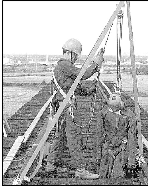
The MSA Bridge Rescue Frame is designed as a portable emergency anchorage for retrieval of railway bridge workers from below the bridge deck. In most cases, the worker cannot be lowered, therefore the anchor point must be above the level of the bridge deck and positioned in such a way that retrieval is possible.
